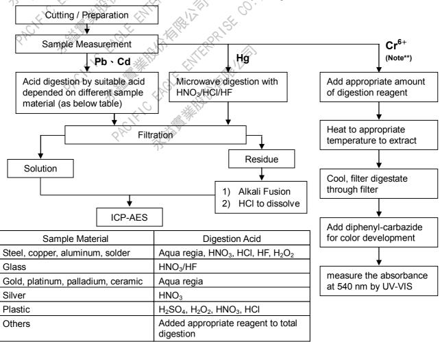
**Note\*\***: (1) For non-metallic material, add alkaline digestion reagent and heat to 90~95℃.
